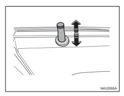
All doors, except the driver's door, can be locked from the outside by pushing down the manual door lock and then closing the door. The driver's door lock cannot be pushed in while the door is open. Upon leaving the vehicle, the driver's door can only be locked from the outside by using the key or the optional remote keyless entry transmitter.
